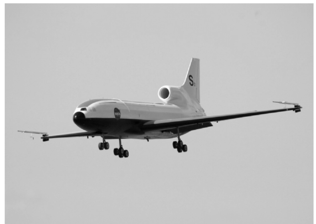
Fig. 2 S-2 subscale jet transport aircraft.
